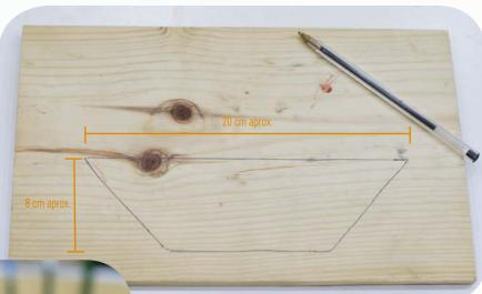
Hammer some nails around the trapezium except the top line. With 15 or 20 nails will be enough to support the weight of the structure.
