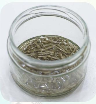
Mix the pieces of rope soaked with moulding compound and knead for a few minutes. The aim of the rope is to avoid cracking upon drying.
